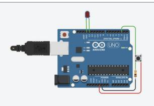
(Descriptive text: Image showing an Arduino board with wires connecting to a pushbutton and a red LED.)
