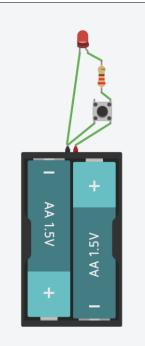
(Descriptive text: Image showing a simple circuit with a red LED, two green wires, a battery pack, and a resistor and a switch. The LED is lit.)
