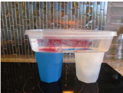
Repeating the experiment, with ice in the white cup. Note how the blue food colour dropped on that side stays flat on the bottom!
