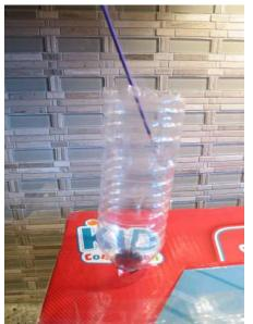
As the smoke is initially hot it has a tendency to rise. If you swish the incense stick around inside the bottle you will notice that a good fraction if it is drawn down into the box and soon comes back out on the other side.
