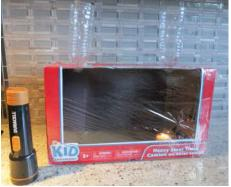
Convection Box, with candle burning on the right. Flashlight can be used to better see the smoke inside. Note that you have to take care to seal ALL cracks and holes other than the two bottles on top. Shining a light at the smoke coming out of the "chimney" at just the right angle is especially helpful.
