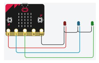
Coding Challenge A. Create a program so that the LEDs light up one after the other.
