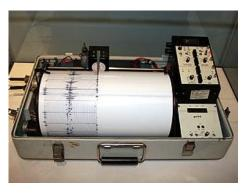
A simple seismometer, sensitive to up-down motions of the Earth, is like a weight hanging from a spring, suspended from a
